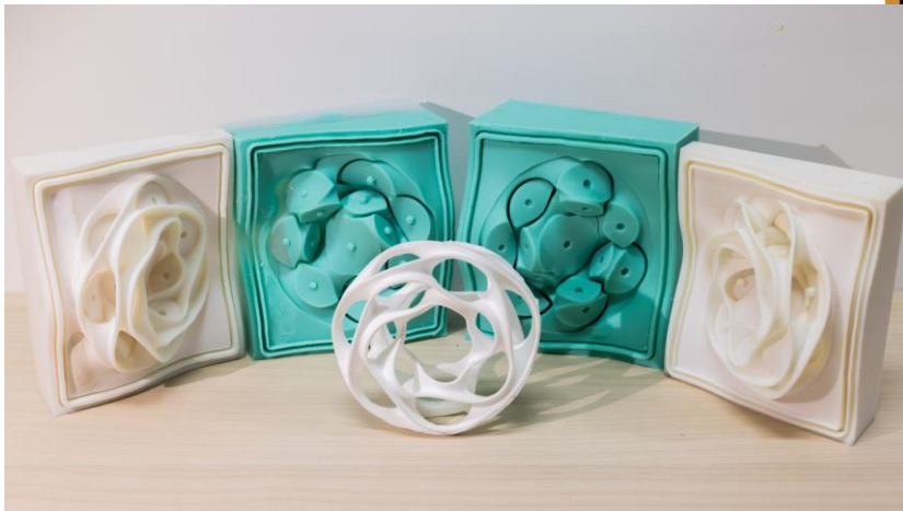
[Metamolds: computational design of silicone molds, Alderighi et al. 2018 ]
